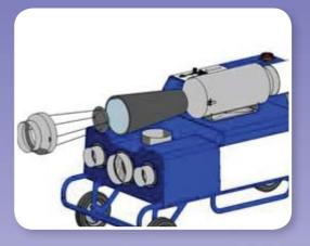
• Interchangeable filter to ensure continued high velocity air replenishment
